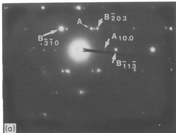
Figure 1 Well-defined epitaxial correlation between two A- and B- \text{Pr}_2\text{O}_3 crystals. (a) Electron diffraction pattern. (b) Drawing of the projection of the two lattices put side by side to illustrate the epitaxy.
